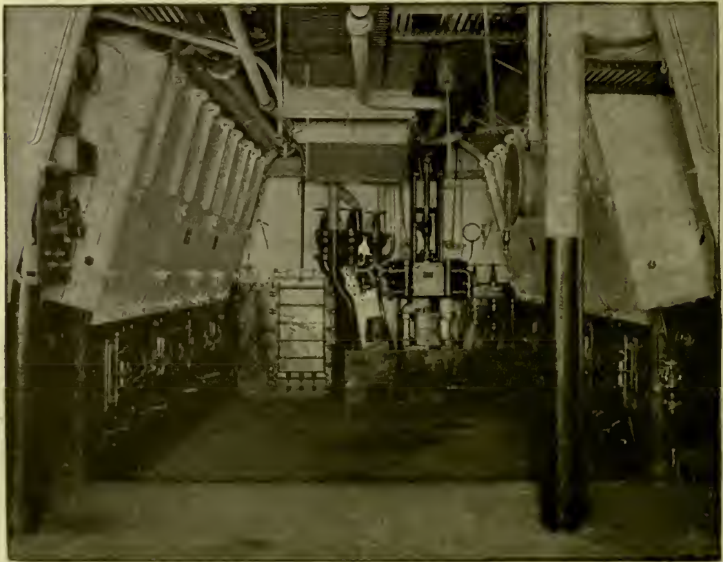
FIRE-ROOM OF A WARSHIP FITTED WITH BABCOCK BOILERS
