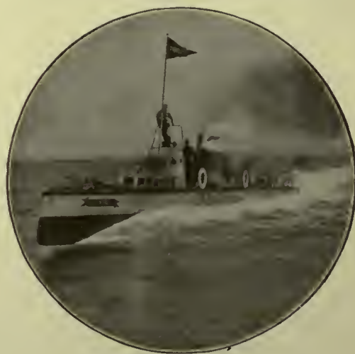
THE "TURBINIA," THE FIRST TURBINE-DRIVEN STEAMBOAT, 1896.
