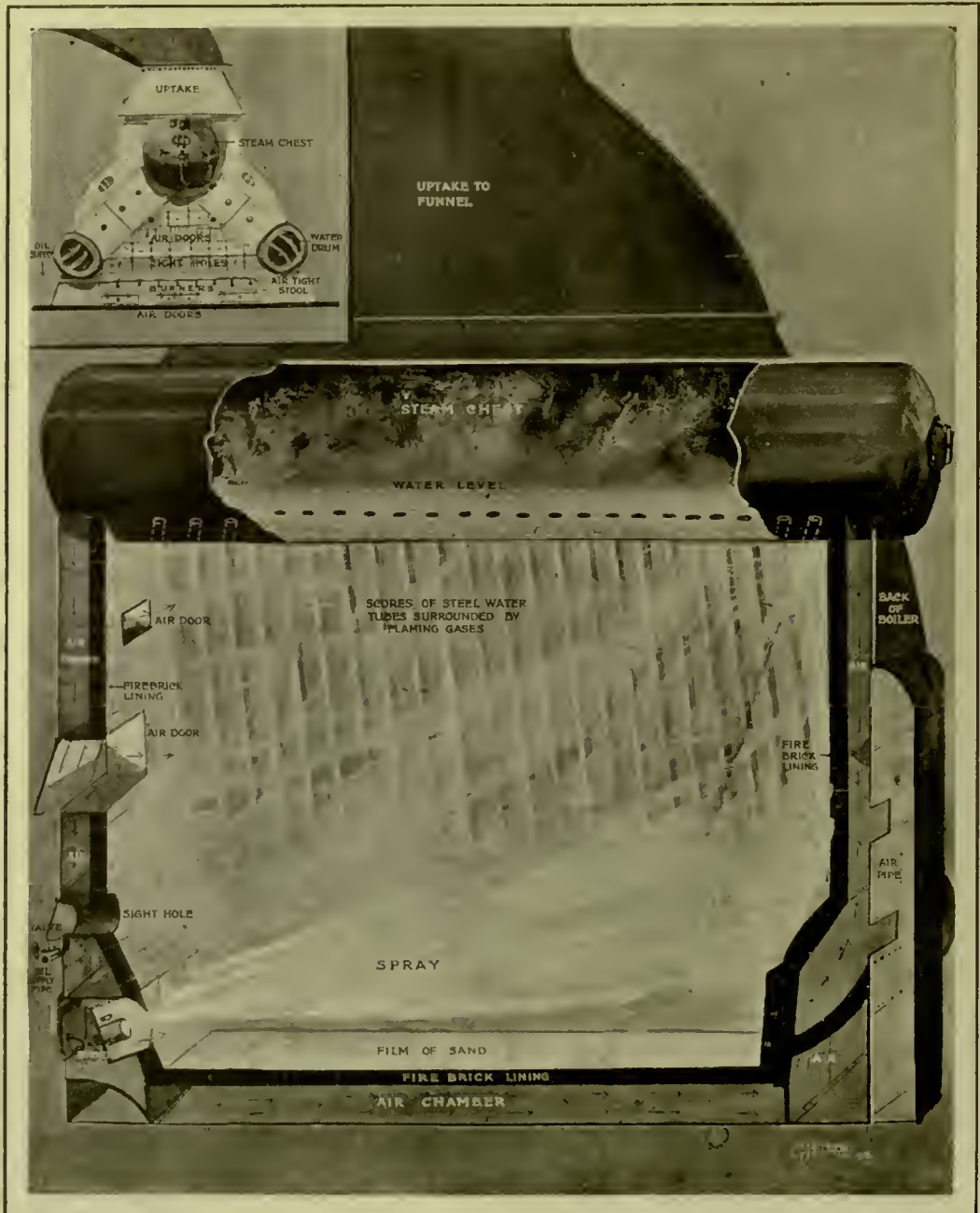
METHOD OF BURNING OIL IN A YARROW BOILER.
