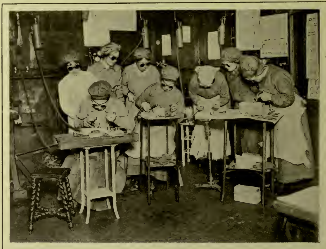
WELDING AEROPLANE PARTS BY MEANS OF ACETYLENE BLOW-PIPES.
