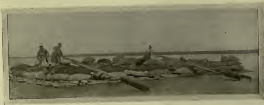
A KELEK OR FREIGHT RAFT ON THE TIGRIS. The raft is buoyed by means of inflated skins beneath the floor of logs.
